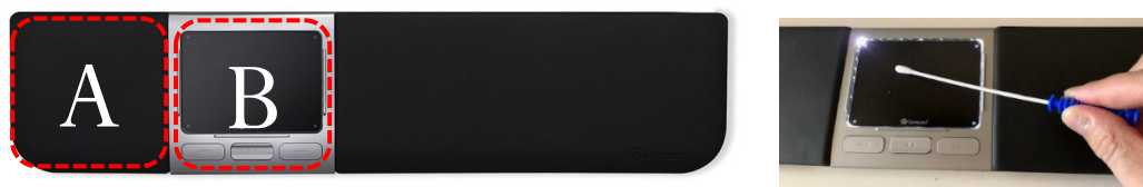
Image 1. Control surfaces. A: Wrist rest left side, 10 x 10 cm. B: Touchpad including buttons, 10 x 10 cm
